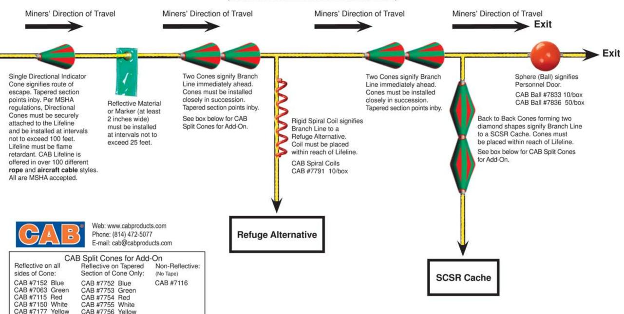
\*Note: CAB Split Cones are identical to standard cones except featuring a pre-engineered hole and slit on one side for easy and secure attachment to lifeline.
