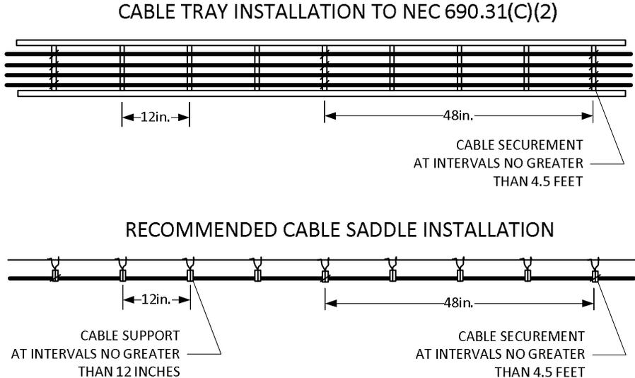
Figure 1: Cable Tray and Cable Saddle Installation Similarities
