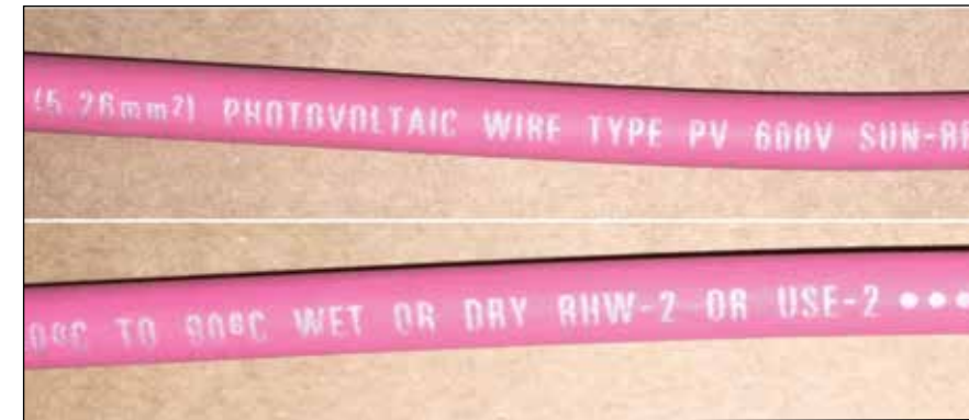
Figure 3. Markings on Listed PV Wire (also listed RHW-2 and USE-2)
